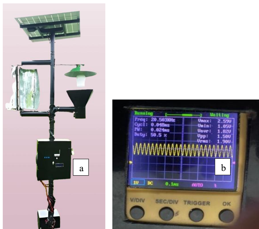
Figure-1. AGRARIS equipment: a. Complete equipment, b. Agraris part that emits ultrasonic waves
