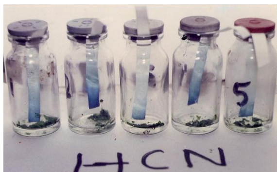
Photograph 1: HCN testing with strips in sealed bottles
